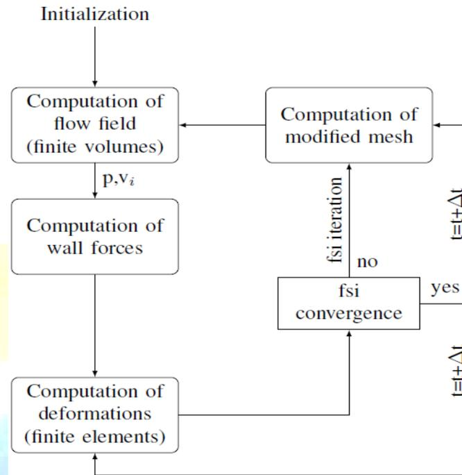
Figure 1: Coupled solution procedure
