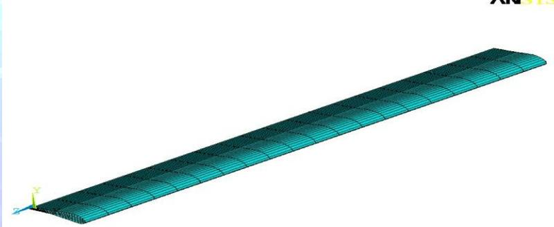
Figure 3: Computational mesh of the wing
