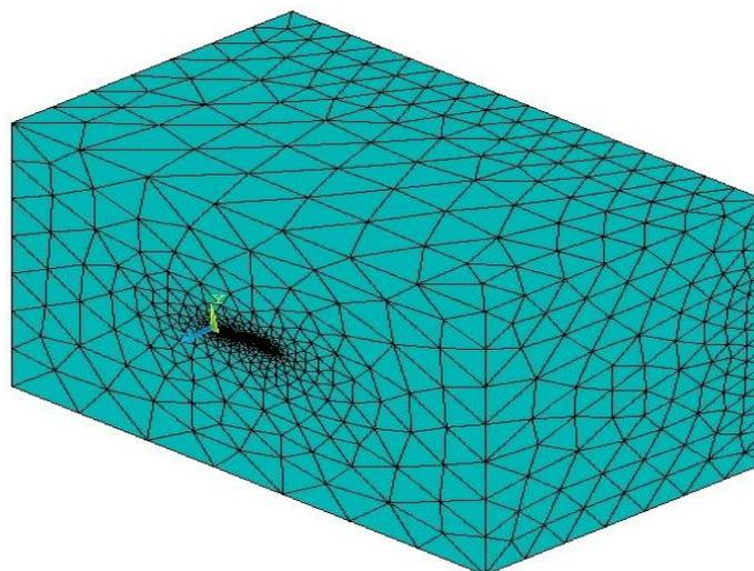
Figure 4: Computational mesh of the fluid domain
