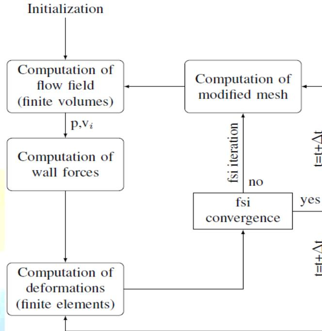
Figure 1: Coupled solution procedure
