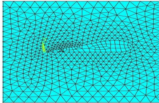
Figure 2: Computational mesh of the two domains
